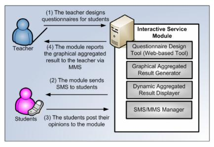
Fig. 2. The communication processes of Interactive Service Module.
